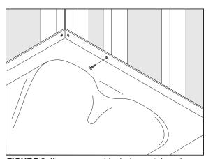
FIGURE 3. If necessary, shim between tub and studs for tight fit and screw to each stud.
